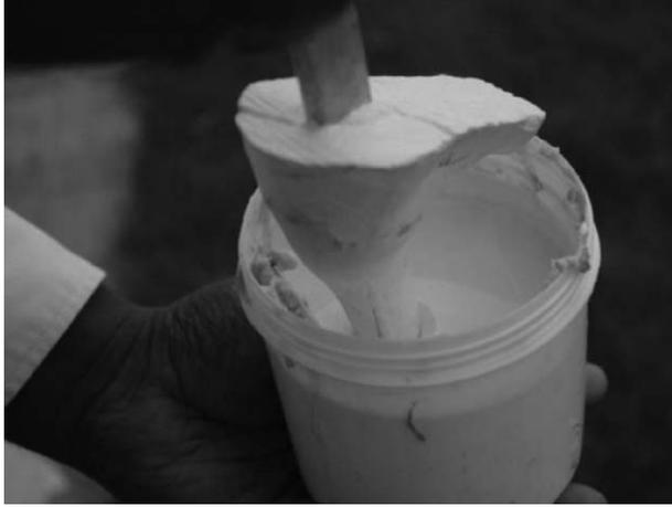
**Figure 5.** Solid POP positive mould being dipped into liquid Latex.
