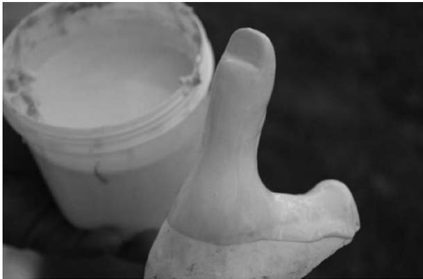
**Figure 6.** Positive mould coated with latex.
